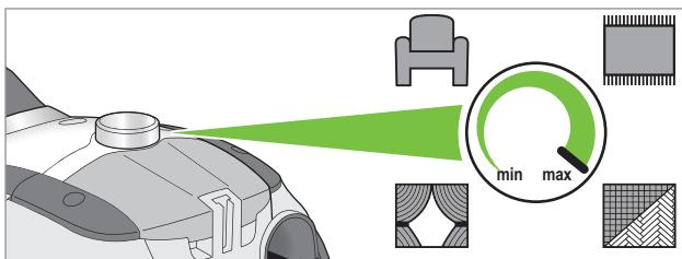
You may steplessly adjust suction power via the power regulator. You should adjust the power regulator position with respect to the floor to be cleaned:
